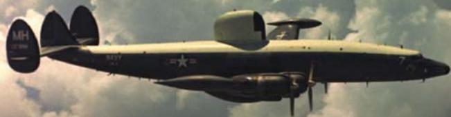
*The WV-3 Warning Star (here, with VW-4, in 1955), the Navy's version of the Lockheed L-1049 Super Constellation, served not only as an airborne early warning platform on radar barrier patrols but also as an effective hurricane hunter.*
