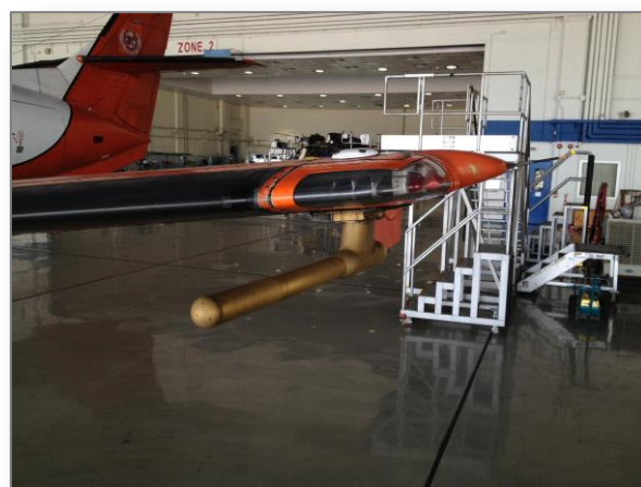
The meteorological probe on the Hong Kong government's SAR aircraft used for Pacific typhoon reconnaissance flights
