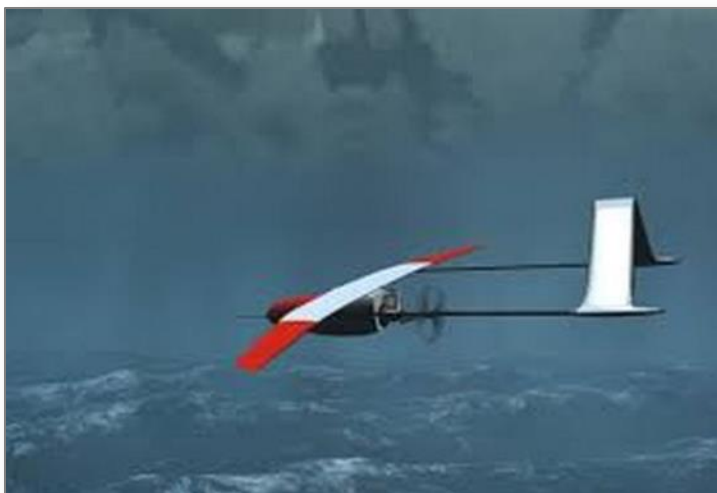
The US Pacific Forces’ WEATHERSCOUT (Aerosonde) UAV, trialed in the Western Pacific as a weather reconnaissance observation platform, which included typhoon surveillance applications in 2005
